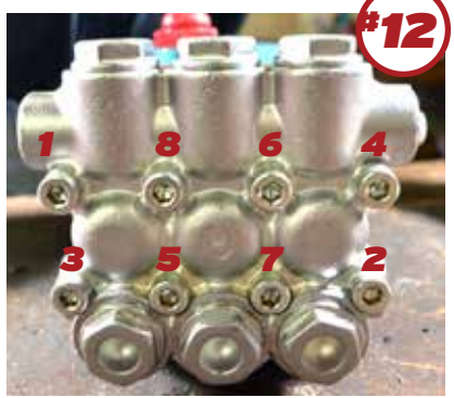
If you don't tighten the head on straight, it could damage the seals. Try to tighten them in this order.
