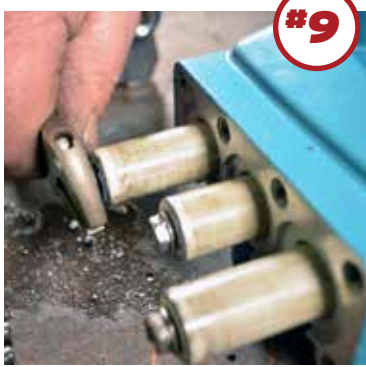
Inspect the ceramic plungers and remove the O-rings on the ends of each plunger.
