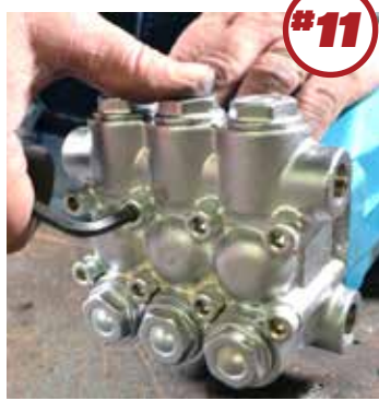
After reinstalling the pump head you will need to tighten the head bolts in a specific order.
