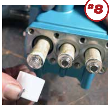
Inspect the seal retainers over the plungers and replace if worn.
