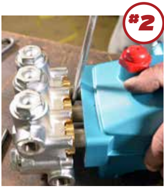
Remove pump head by slowly prying with a large screwdriver. Be careful not to damage anything.
