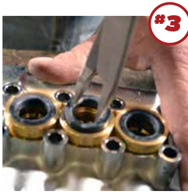
Using the low pressure seals, remove the low pressure seals. Always replace these seals once removed.
