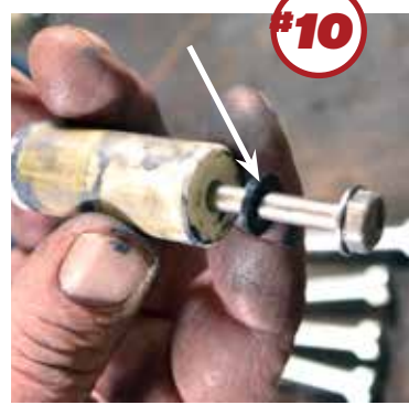
Replace the O-rings that are attached to the end of the plungers.
