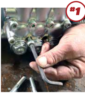
Remove all 8 head bolts with an allen wrench.
